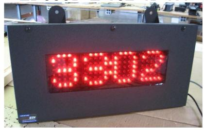
An outdoor rated enclosure. 6" high numbers using outdoor LEDS. Display real-time information to your employees or customers. The display will up-time in MM:SS (default) or HH:MM (select when ordering) when a customer-supplied on/off switch is activated. A separate momentary switch will reset the unit to "00:00".
