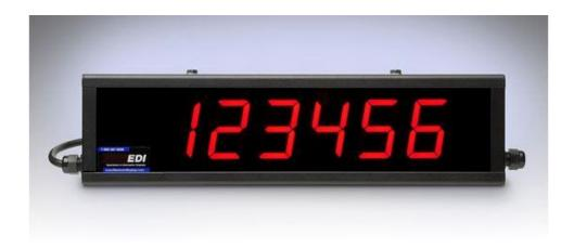
Indoor, Six Digits. Visible up to 90 Feet Away Dimensions: 16"L x 4"H x 2.25"D Display real-time information to your employees or customers. The display will advance by "1" for every activation of a customer-supplied momentary switch. A separate momentary switch will reset the unit to "0". EDI also supplies an on-board 14VDC Power supply.
