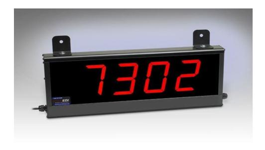
Indoor, 4 digit. Dimensions: 20"L x 8"H x 2.5"D Count up or down. Thumbwheel preset standard. Serial preset available. Two momentary inputs: increment/decrement by 1, preset to value. "Wet" or "Dry" contacts. Photo-eye, limit switch, etc. Ideal for assembly line production.
