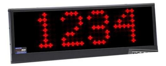
Indoor, 4 digit. Dimensions: 26"L x 9.4"H x 3"D. Keypad provided to preset the display. Display real-time production information to your employees or customers. The display will up-count or down-count by one when a customer-supplied on/off switch is activated. A separate momentary switch will preset the unit to a value designated from a remote keypad (included).
