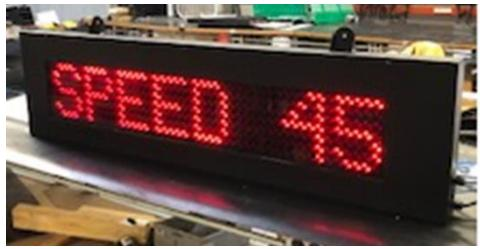
Dimensions: 37" x 11" x 3" Display real-time information to your employees or customers. Display real-time information to your employees or customers. The display will receive data from an PLC through an EIP gateway. The EIP gateway (ED3600) is built in the enclosure. Works with A/B Studio 5000.
