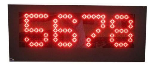
Dimensions: 51" x 21" x 4" Display real-time information to your employees or customers. The display will advance by "1" for every activation of a customer-supplied momentary switch. A separate momentary switch will reset the unit to "0". EDI also supplies an on-board 14VDC Power supply.
