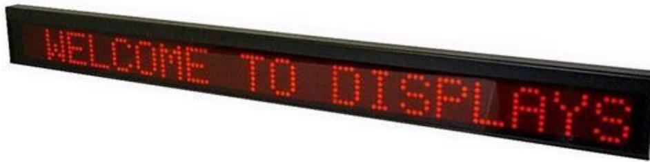
Displays are used to loaded status messages for the production lines. Customer selected messages will be triggered by BCD to display machine status or part status.
