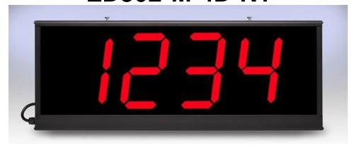
Visible up to 380 feet Dimensions: 36" L x 11.5" H x 2.25" D. Display real-time information to your employees or customers. The display will receive data from an PLC through a Modbus gateway. The Modbus gateway (ED3600M)is built in the display.
