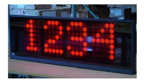
Visible up to 575 Feet Away. Dimensions: 52"L x 17.7"H x 3.5"D Display real-time information to your employees or customers. The display will advance by "1" for every activation of a customer-supplied momentary switch. A separate momentary switch will reset the unit to "0". EDI also supplies an on-board 14VDC Power supply.
