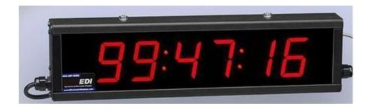
Dimensions: 28" L x 8" H x 2.25" D. Display real-time information to your employees or customers. The display will down-time in HH:MM:SS (default) when a customer-supplied on/off switch is activated. A separate momentary switch will reset the unit to "00:00:00. Keypad included to preset a time
