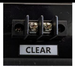
A 'Clear' terminal block has been added to the EDV225MPC-2L-N1-GR-IR. A contact closure between the two terminals will reset the second (Actual) line of the display. Reset occurs after contact between the two terminals is released.
