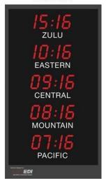
GSA Contract GS-02F-0134V Bright 2.25" High LED Display with Eight Time Zone Fields Dimensions: 50"H x 15"W x 3"D White, vinyl location designators under each time zone HH:MM in Military Time Format. Mounting Brackets
