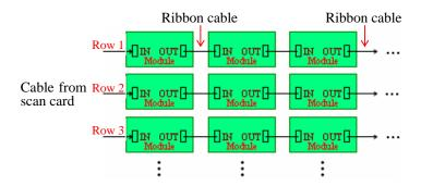
Fig4.1 LED modules connection(I)
