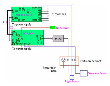
Fig4.6 TCP/IP connection in sign
