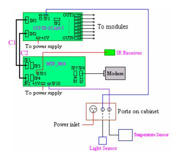
Fig4.5 Modem connection in sign
