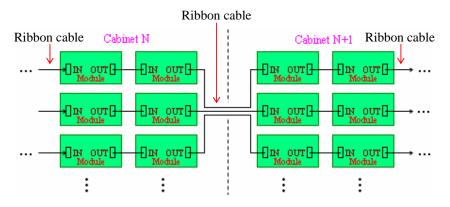
Fig4.2 LED modules connection(II)
