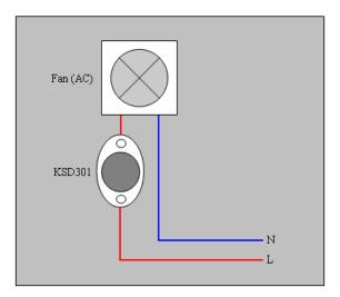
Fig3.1 Fans connection diagram
