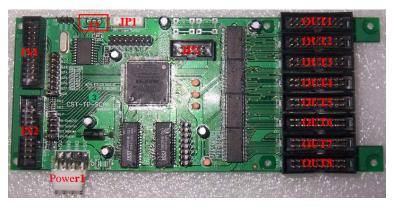
Fig1.2 Scan card (CST-TP-SCAN-C)
