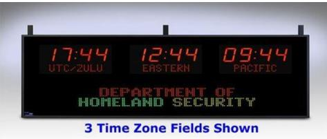
Five Field Time Zone Display with Digital Lettering. 2.25" high numbers for time and 1.6" High Alphanumeric lettering for Location. Two-line moving message sign with IR remote.
