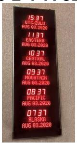
Display time / location and date. The horizontal series time zone displays have bar segment time displays with a ten-character dot matrix digital zone label below. The digital zone labels can hold any ASCII test string and is independent of the time zone parameters. Every display includes a high accuracy crystal oscillator and your choice of Ethernet, USB or RS232 interface for time zone parameter control
