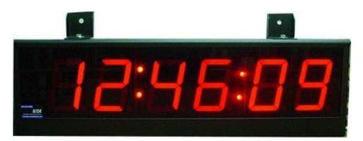
Dimensions: 26"L x 8"H x 2.25"D . The clock includes two push buttons on the end cap are used for fast set and slow set. A terminal block inside the display can be used to wire in remote switches.
