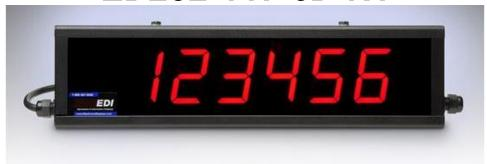
Indoor, Six Digit, Visible up to 90 Feet Away Dimensions: 16" L x 4" H x 2.25" D. Display real-time production information to your employees or customers. The display will receive an RS422/RS485 data signal from a PC / PLC and update the unit using standard ASCII protocol.
