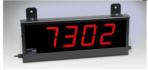
This four digit model receives a customer supplied BCD input and displays it. Weights 1, 2, 4 and 8 are common for all four digits. "Common" and strobes are also common (six wires per digit).
