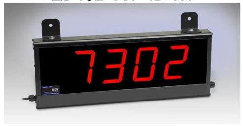
Visible up to 190 feet Dimensions: 20" L x 8" H x 2.25" D. Display real-time production information to your employees or customers. The display will receive an RS422/RS485 data signal from a PC / PLC and update the unit using standard ASCII protocol.
