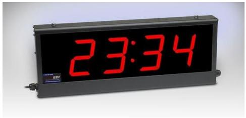
Dimensions: 16" L x 4.0" H x 2.25" D. A 4-digit up and/or down timer with internal timing in MM:SS (minutes-seconds) or HH:MM (hours-minutes) format standard. Other time formats available. The display is preset via thumb wheel switches on the end plate or keypad remote (optional).
