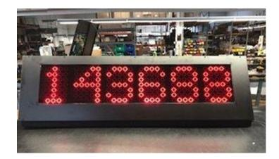
Dimensions: 81" x 18.25" x 4" Display real-time information to your employees or customers. The display will advance by "1" for every activation of a customer-supplied momentary switch. A separate momentary switch will reset the unit to "0". EDI also supplies an on-board 14VDC Power supply.
