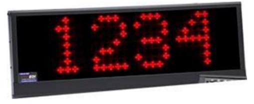
Visible up to 280 feet Indoor, 4- digit, Dimensions: 26" L x 9.4" H x 3" D. Display real-time production information to your employees or customers. The display will receive an RS422/RS485 data signal from a PC / PLC and update the unit using standard ASCII protocol.
