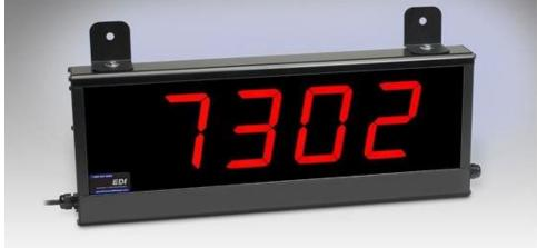
This four-digit model receives a customer supplied BCD input and displays it. Weights 1, 2, 4 and 8 are isolated (four wires per digit). Strobe and "common (negative return)" are common for all digits.
