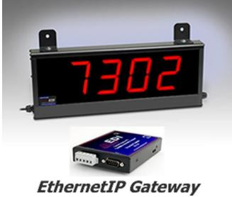
Dimensions: 26" L x 8" H x 2.25" D. Display real-time information to your employees or customers. The display will receive data from an PLC through an EIP gateway. The EIP gateway (ED3600) is built in the display. Works with A/B Studio 5000 and many more.
