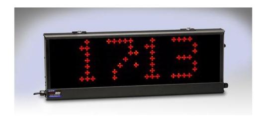
8" High Numbers! LED Display with Four Digits Programmed using a detachable Keypad. Up or down-timer in MM:SS or HH:MM format (others available) Two Contact closures - run / hold and preset.
