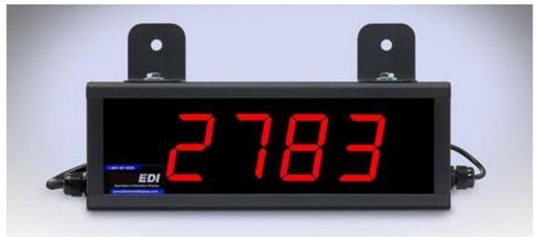
Indoor, Four Digit, Visible up to 90 Feet Away Dimensions: 12" L x 4" H x 2.25" D. Display real-time production information to your employees or customers. The display will receive an RS422/RS485 data signal from a PC / PLC and update the unit using standard ASCII protocol.
