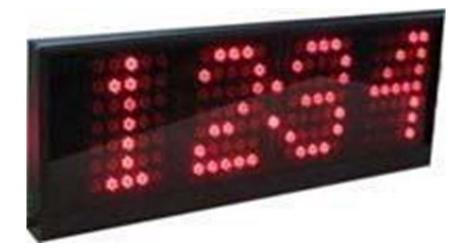
12" High Numbers! LED Display with Four Digits Programmed using a detachable Keypad. Up or down-timer in MM:SS or HH:MM format (others available) Two Contact closures - run / hold and preset.
