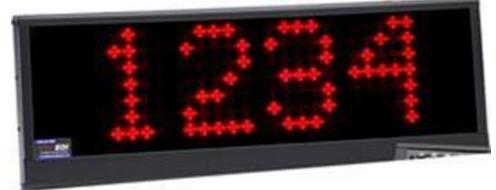
Up To 12 Digits Available. Indoor, 4- digit, Dimensions: 26" L x 9.4" H x 3" D. Display real-time production information to your employees or customers. The display will receive an RS232 data signal from a PC / PLC and update the unit using standard ASCII protocol.
