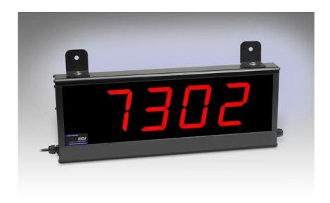
Viewable up to 200 Feet Away. Dimensions: 2"L x 8"H x 2.5"D Display real-time information to your employees or customers. The display will advance by "1" for every activation of a customer-supplied momentary switch. A separate momentary switch will reset the unit to "0". EDI also supplies an on-board 14VDC Power supply.
