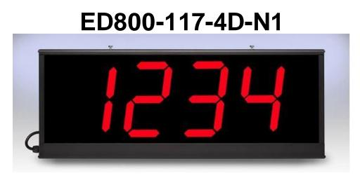
Indoor, 4- digit, Dimensions: 36" L x 14" H x 3" D. Display real-time production information to your employees or customers. The display will receive an RS422/RS485 data signal from a PC / PLC and update the unit using standard ASCII protocol.
