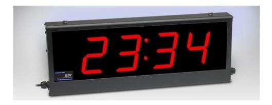
Dimensions: 20" L x 8.0" H x 2.25" D. A 4-digit up and/or down timer with internal timing in MM:SS (minutes-seconds) or HH:MM (hours-minutes) format standard. Other time formats available. The display is preset via thumb wheel switches on the end plate or keypad remote (optional).
