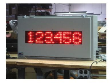
Dimensions: 30" x 16" x 6" Display real-time information to your employees or customers. The display will advance by "1" for every activation of a customer-supplied momentary switch. A separate momentary switch will reset the unit to "0". EDI also supplies an on-board 14VDC Power supply.
