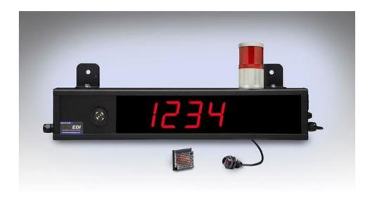
4 digit. Dimensions: 20"L x 4"H x 2.25"D Count up or down. Thumbwheel preset standard. Serial preset available. Two momentary inputs: increment/decrement by 1, preset to value. "Wet" or "Dry" contacts. Photo-eye, limit switch, etc. Ideal for assembly line production. Audible output and tower light activated when the display reaches "0".
