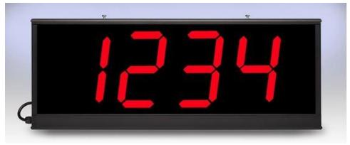
Visible up to 380 feet Dimensions: 36" L x 11.5" H x 2.25" D. Display real-time information to your employees or customers. The display will receive data from an PLC through an EIP gateway. The EIP gateway (ED3600) is built in the display. Works with A/B Studio 5000 and many more.
