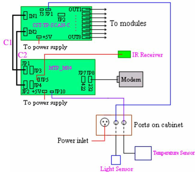
Fig4.5 Modem connection in sign
