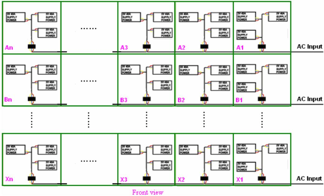
Fig2.2 Example for power supply connection
