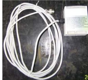
Fig1.5 Temperature sensor
