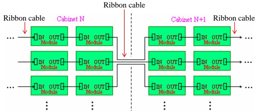
Fig4.2 LED modules connection(II)
