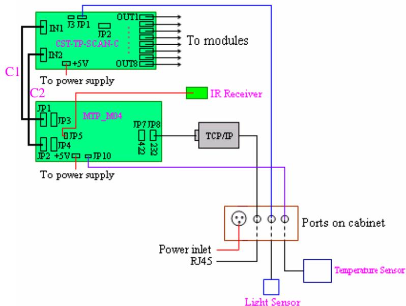
Fig4.6 TCP/IP connection in sign
