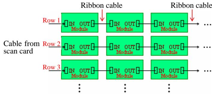
Fig4.1 LED modules connection(I)
