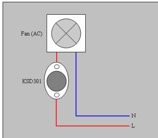
Fig3.1 Fans connection diagram
