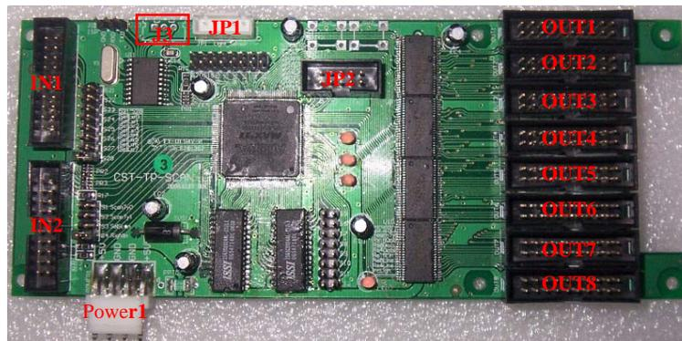
Fig1.2 Scan card (CST-TP-SCAN-C)
