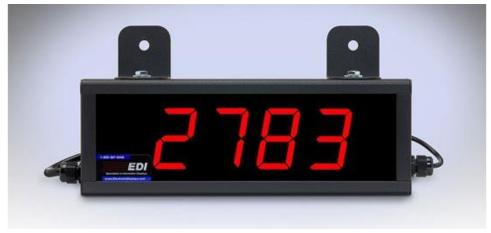
Visible up to 90 feet Dimensions: 16" L x 8" H x 2.25" D. Display real-time information to your employees or customers. The display will receive data from an PLC through a Profinet gateway. The gateway (ED3600-P) is built in the display.
