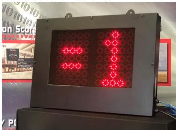
Visible up to 575 feet Dimensions: 30" L x 21.5" H x 3" D. Display real-time information to your employees or customers. The display will receive data from an PLC through an EIP gateway. The EIP gateway (ED3600) is built in the enclosure. Works with A/B Studio 5000.
