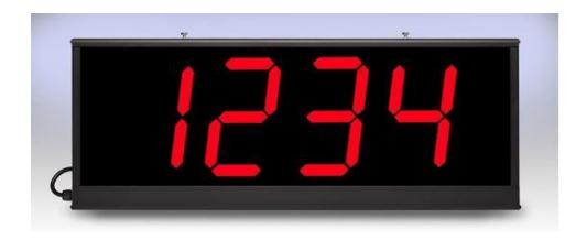
Indoor, 4 digit. Dimensions: 36"L x 11.4"H x 3"D. Keypad provided to preset the display. Display real-time production information to your employees or customers. The display will up-count or down-count by one when a customer-supplied on/off switch is activated. A separate momentary switch will preset the unit to a value designated from a remote keypad (included).
