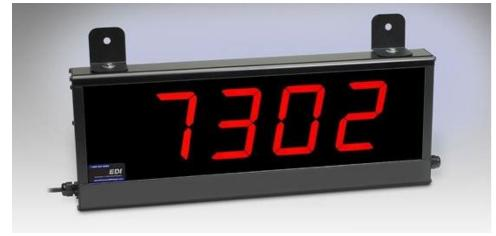
This four digit model receives a customer supplied BCD input and displays it. Weights 1, 2, 4 and 8 and commons are isolated (five wires per digit). There are no strobe inputs.
