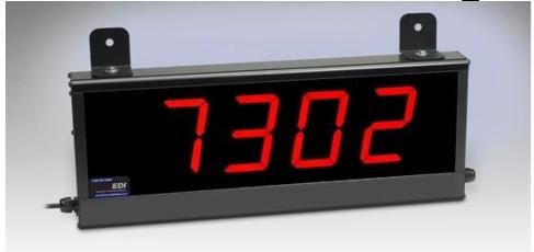
This four-digit model receives a customer supplied BCD input and displays it. Weights 1, 2, 4 and 8 are common for all four digits. "Common" and strobes are isolated (five wires per digit).
