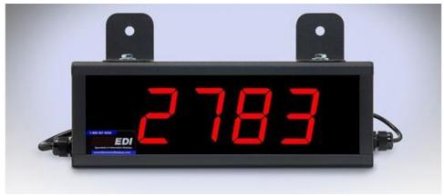
Visible up to 90 Feet Away. Dimensions: 12"L x 4"W x 2.25"D Convert your analog signal for temperature, speed, weight measurements to a large digital display. Standard analog inputs include: 4 to 20 mA or 0 to 10VDC. Others Available Upon Request.
